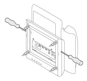
The following diagram shows how to disengage the locking tabs on the Cisco IP Phone 8800 series with a key expansion module attached.
