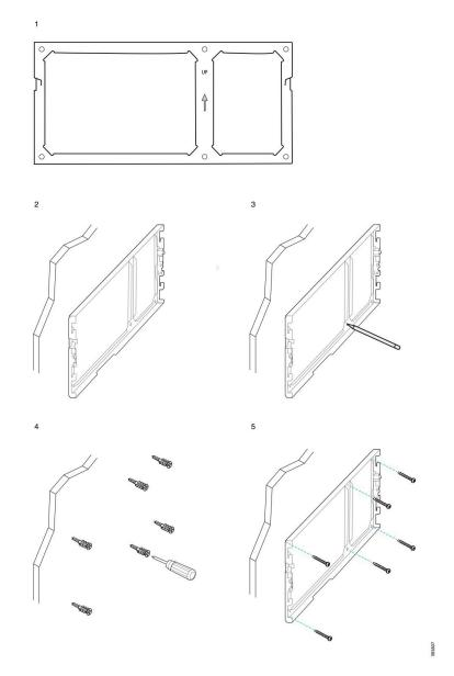
The following diagram illustrates attaching a Cisco IP Phone 8800 series wall bracket with a key expansion module to a wall.
