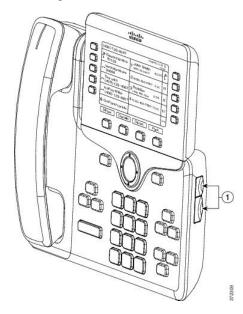
**Step 4** Remove the two accessory connector covers, as shown in the diagram.
