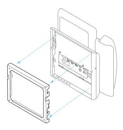
The following diagram illustrates how to attach a Cisco IP Phone 8845 and 8865 to your wall bracket.
